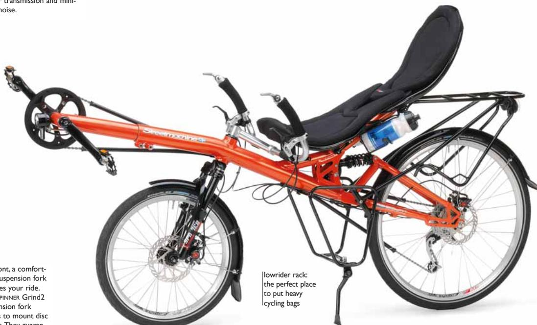
Up front, a comfortable suspension fork soothes your ride. The *SPINNER Grind2* suspension fork allows to mount disc brakes. They guarantee incredible braking performance when going downhill.
